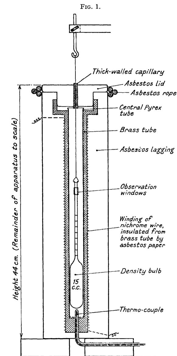
$\times \frac{1}{4}$  cm.), and a central Pyrex-glass lining which prevents any possible local cooling effect by these apertures.
